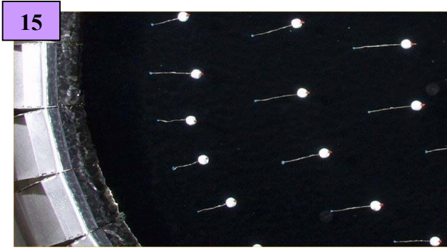
15. Tethered sub-surface wooden balls create their own turbulence but give quick guide to flow 16. Red: still water. Superimposed yellow, green & blue photos show 120 degree rotation of flow 17. Red-blue vectors show simple \sin(x) flow. 18. \sin(2x) cam profile gives simplest contra-flow
