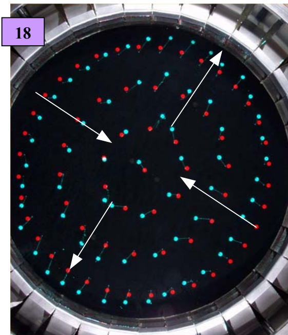
15. Tethered sub-surface wooden balls create their own turbulence but give quick guide to flow 16. Red: still water. Superimposed yellow, green & blue photos show 120 degree rotation of flow 17. Red-blue vectors show simple \sin(x) flow. 18. \sin(2x) cam profile gives simplest contra-flow
