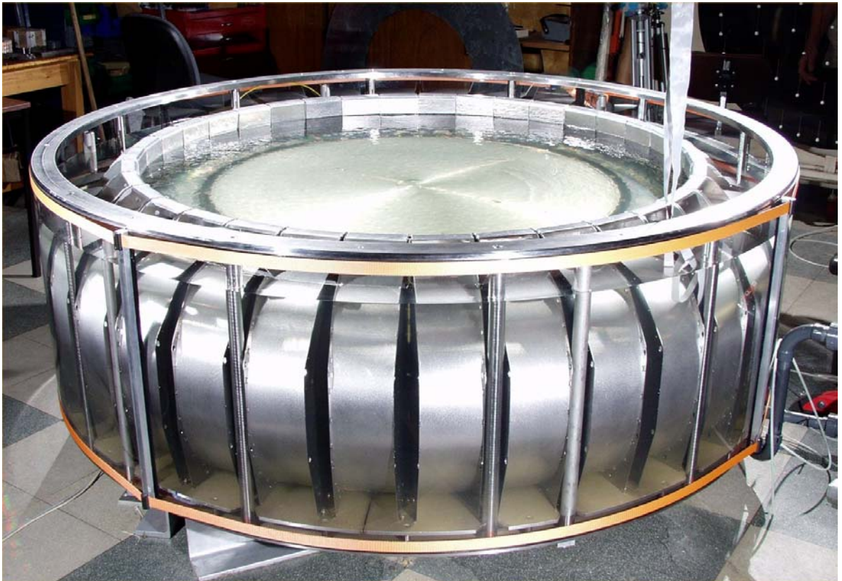
Photo 2: Flow table complete and filled with water. The outer rim is the same height as a billiard table. The water can be quickly transferred to or from an adjacent storage tank.
