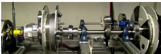
Figure 4: A more detailed view of the converter. The anchor drum can be seen to the right, and the planetary gear and generator to the left.
