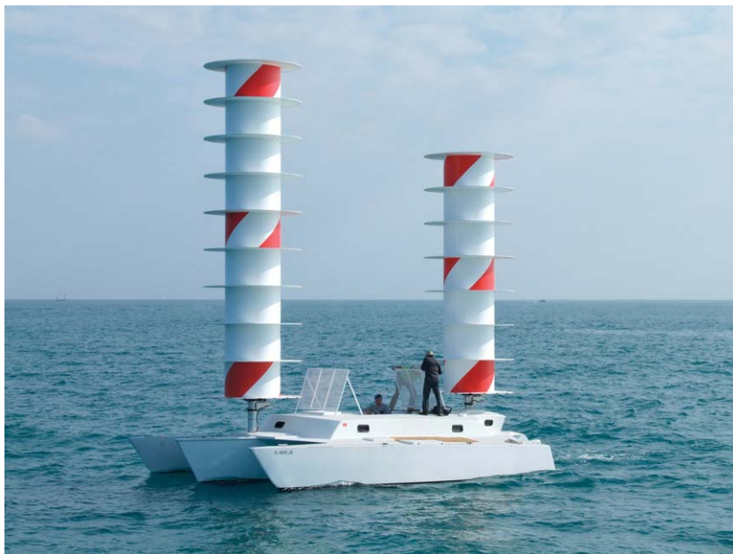
Figure 7. John Marples' Cloudia (a rebuilt Searunner 34 ), with Thom fences on test at Fort Pierce, FL, February 2008. With a rotor drive power of 600 watts, she could sail faster than the beam wind, stop, go into reverse and yaw 180^\circ in either direction about her own axis. Funding for work on Cloudia was provided by the Discovery Channel and organized by Impossible Pictures. © Discovery Channel.
