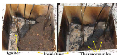
Figure 4 – Small-scale experiments in 100 x 100 mm samples. Snapshots of peat front propagating (time elapsed is ~1 h).
