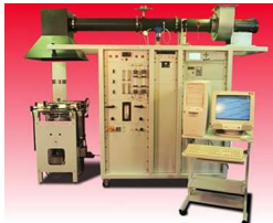
Figure 2. FM Global's Fire Propagation Apparatus (FPA). This calorimeter enables for different external heat fluxes and different flow condition to be applied on the samples.
