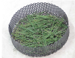
Figure 3. Sample Holder with live needles. The Edinburgh porous sample holder used here and developed in [1]
