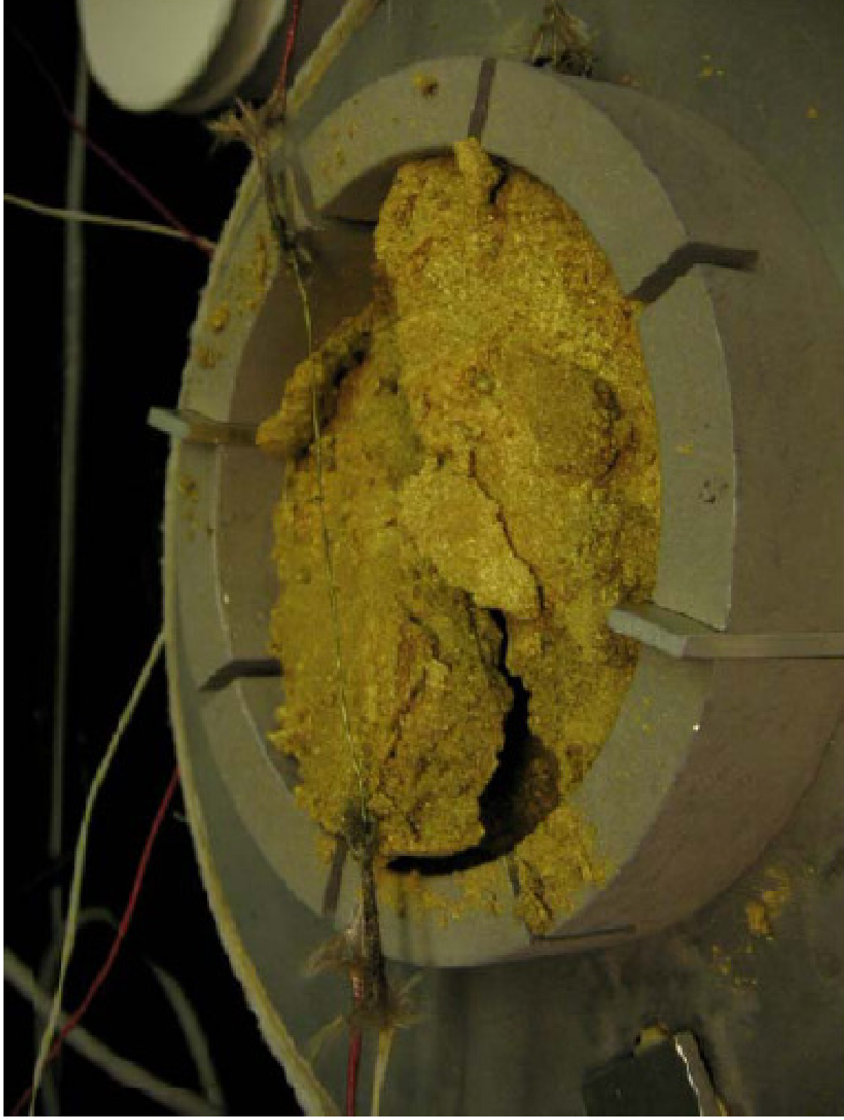
Figure 70 : At the end of test of brass powder with 4% stearic acid at 400 °C
