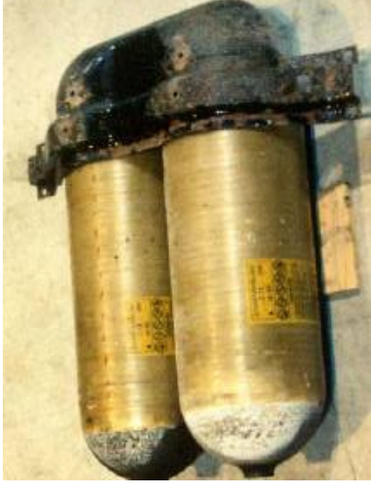
Type 2: Hoop-wrapped composite (fiber + resin) with thick metal liner
