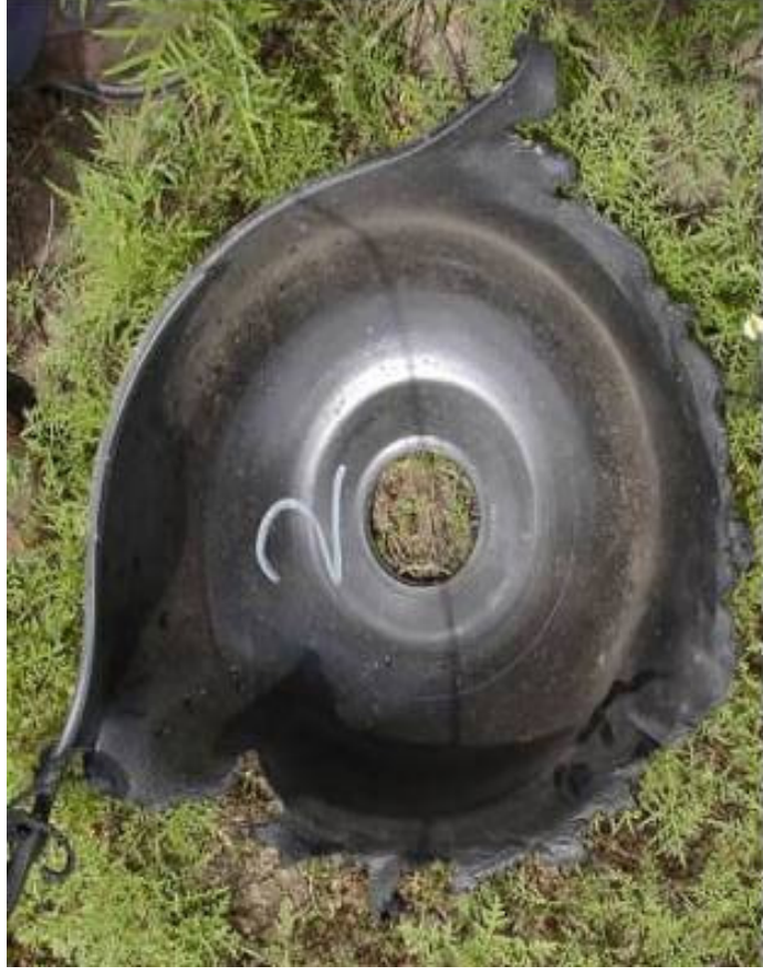
Cylinder dome 2 kg end cap projectile
